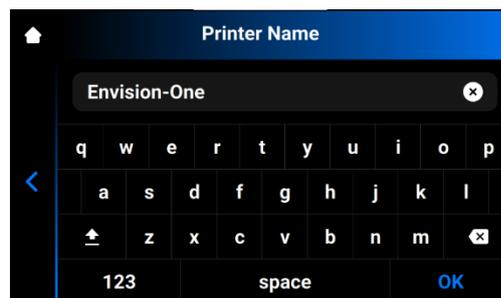
2. Enter the required name of the printer into the corresponding field using the keyboard on the screen.
