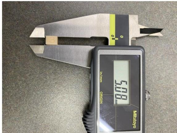
Figure 10: Measuring calibration cube with the caliper
