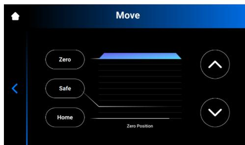
2. Select the **Up** and **Down** arrows to move the platform up and down correspondingly.
